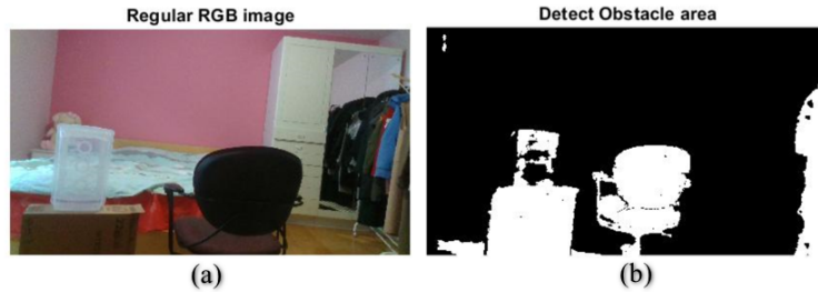
Figure 2.3: Obstacle detected in depth field
